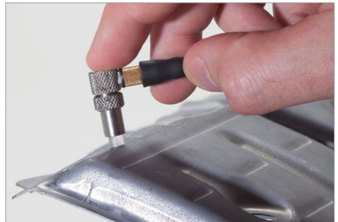
Measure metal thinning caused by bending or forming.
