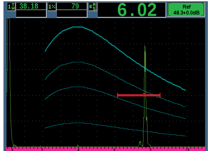
EPOCH 650 DGS/AVG feature—full screen mode
