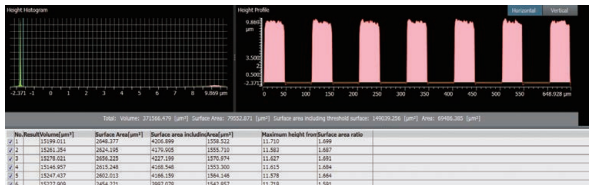
Metal bump / Joint uniformity (Height evaluation) (MPLAPON20XLEXT)
