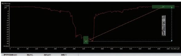
Corrosion on stainless steel / Height measurement (MPLAPON20XLEXT / 3 × 3 stitched)
